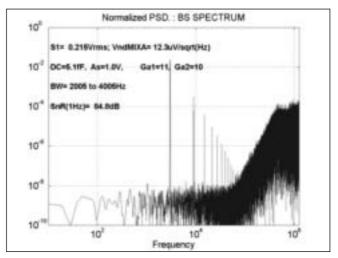
Figure 6: Spectrum at the output of the modulator (BS)
