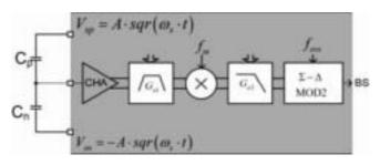
Figure 2: Architecture of the ASP circuit
