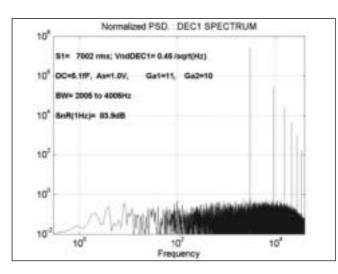
Figure 7: Spectrum at the output of the DEC1
