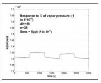
Figure 11: Measured response of the sensor
