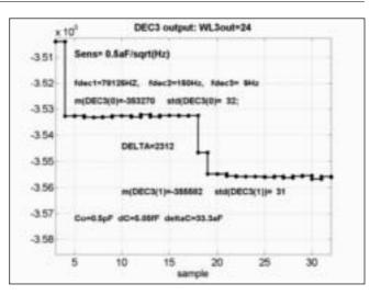
**Figure 9:** Response at DEC3 output to  $\Delta C_0 = 5 fF$  and  $\delta C = 33 aF$
