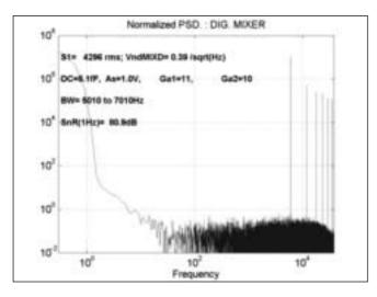
Figure 8: Spectrum after digital mixer
