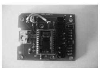
Figure 10: PCB with sensors and ASIC
