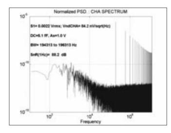
**Figure 4**: Output spectrum of CHA for  $\Delta C = 5 fF$
