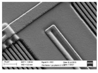
Figure 1: SEM of differential COMB sensor
