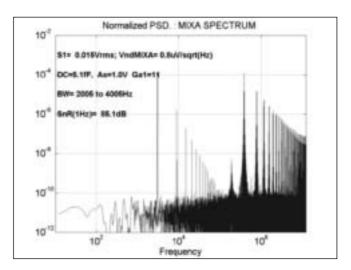
**Figure 5:** Spectrum at the output of passive mixer for A = 1V and  $\Delta C = 5 fF$   $G_{a1} = 11$
