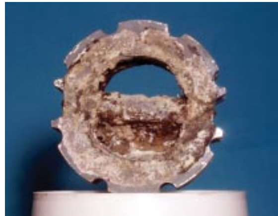
Amalgam waste on a vacuum line valve from a dental clinic. Medical Photography Department, Naval Health Clinic, Great Lakes, IL
